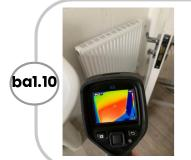
The radiator appears to need bleeding as the top of the radiator's output from the top is not as strong, suggesting an air
