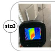
The radiator appears to need bleeding as the top of the radiator's output from the top is not as strong, suggesting an air pocket
